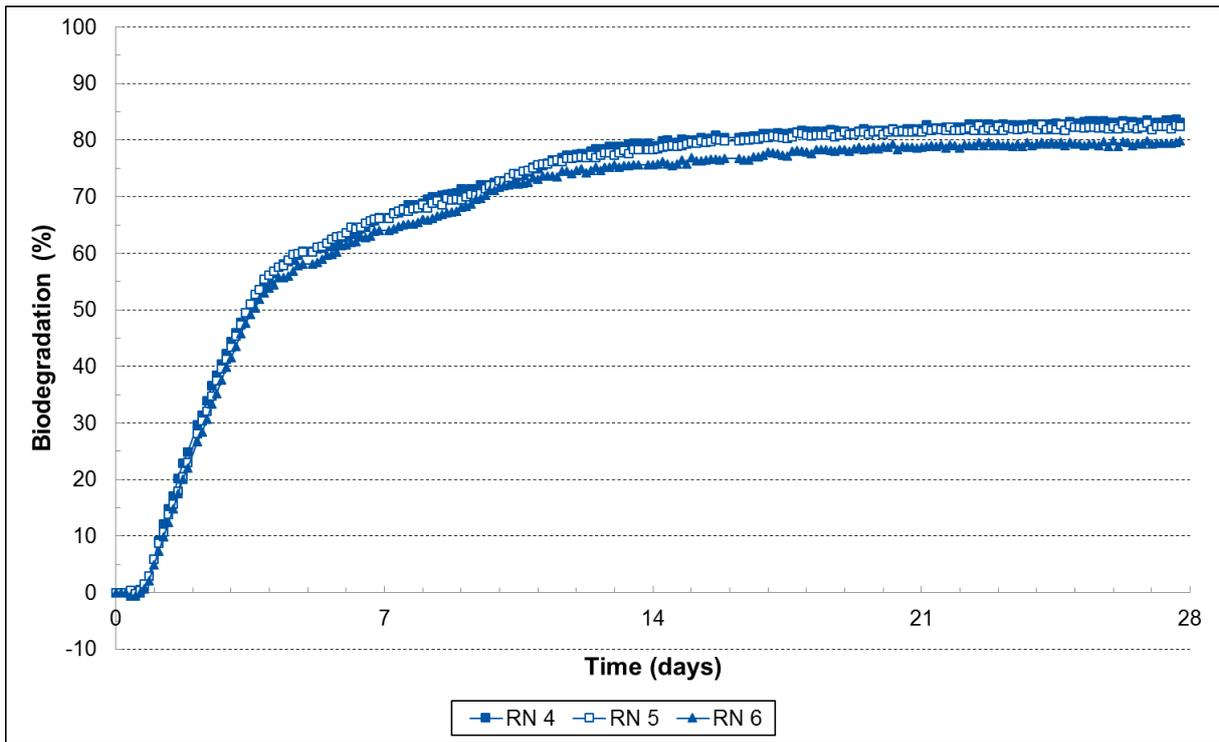
Figure 6. Evolution of the biodegradation percentage of replicates of cellulose (based on O<sub>2</sub> consumption)
