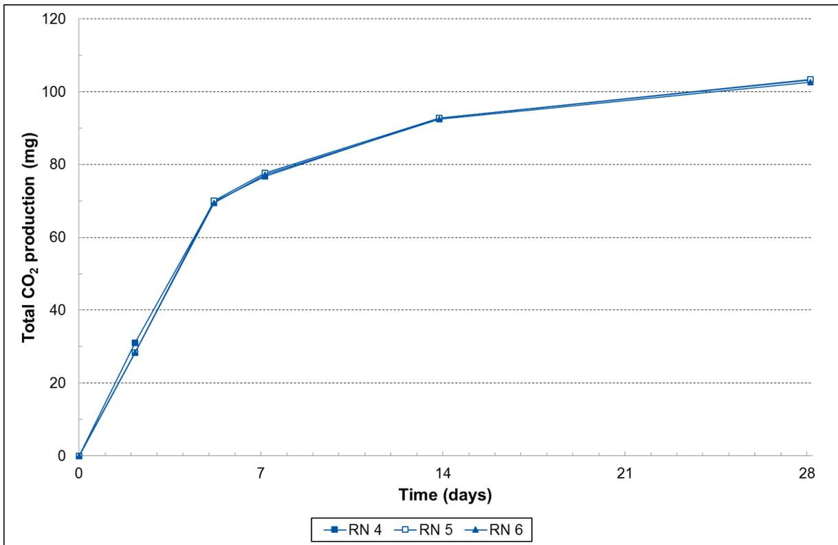
Figure 9. Evolution of the cumulative CO<sub>2</sub> production of the cellulose reactors
