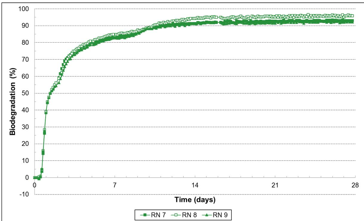
Figure 7. Evolution of the biodegradation percentage of replicates of NuPlastiQ GP 1000 (based on O<sub>2</sub> consumption)
