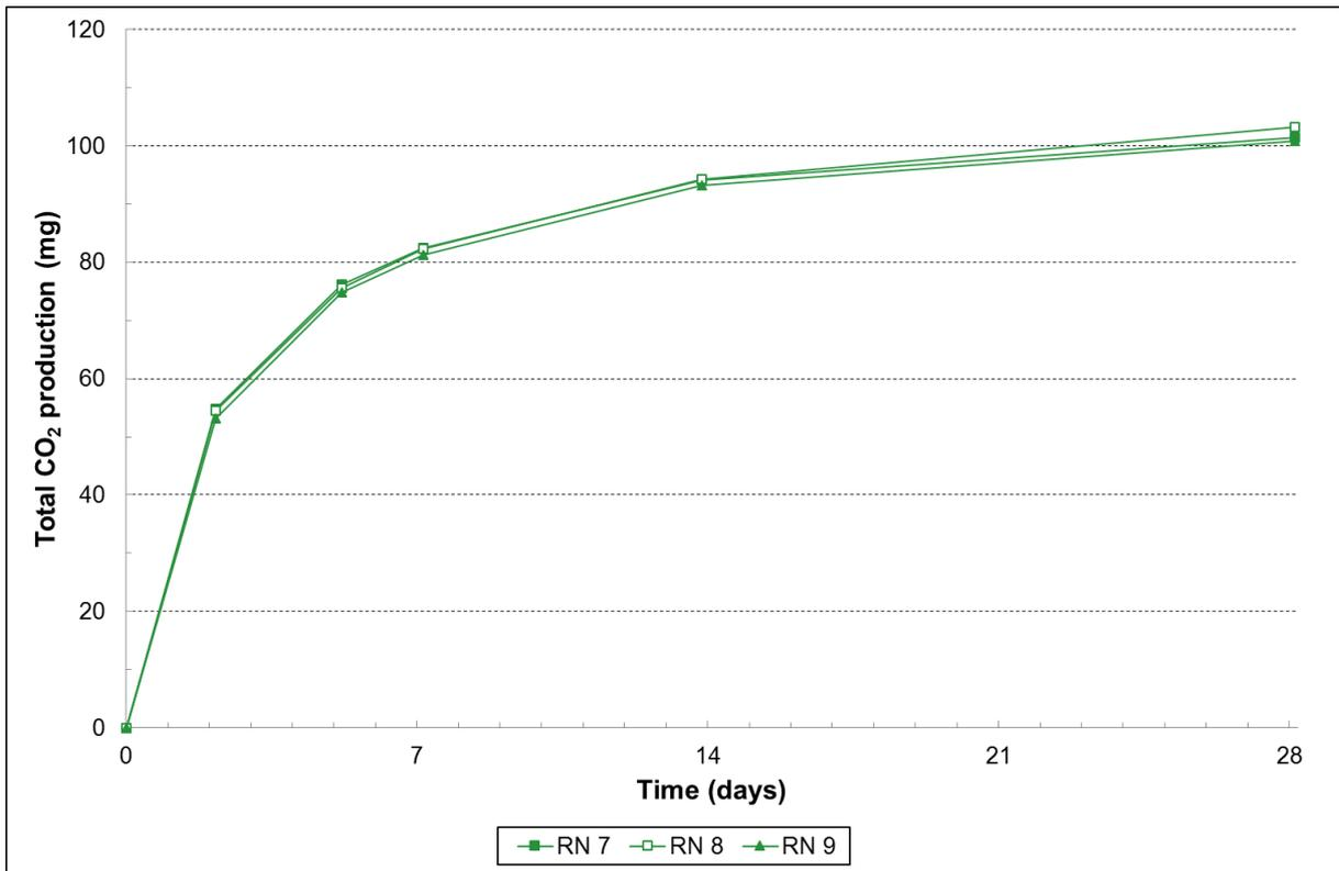
Figure 10. Evolution of the cumulative CO<sub>2</sub> production of the NuPlastiQ GP 1000 reactors
