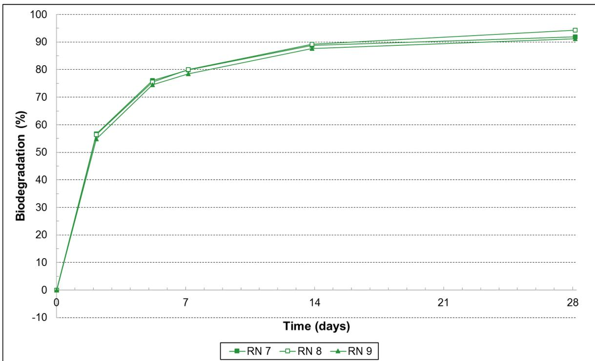
Figure 13. Evolution of the biodegradation percentage of replicates of NuPlastiQ GP 1000 (based on CO<sub>2</sub> production)
