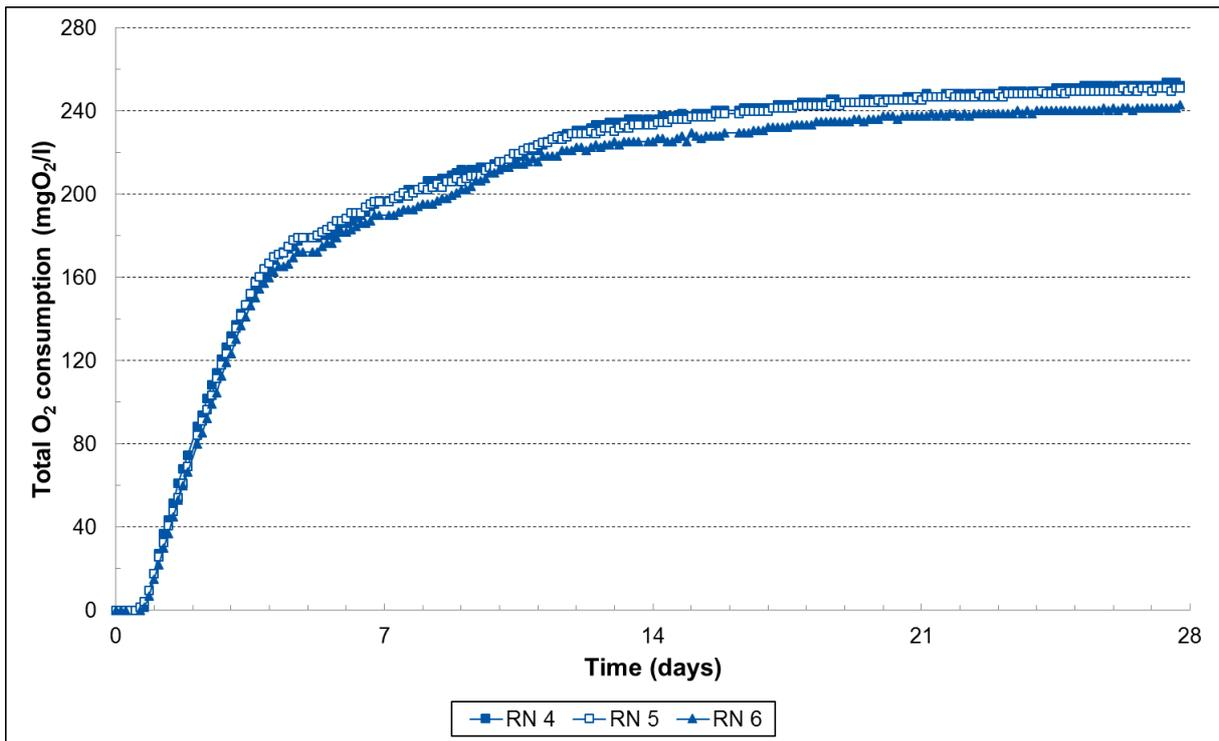
Figure 3. Evolution of the cumulative O<sub>2</sub> consumption of the cellulose reactors
