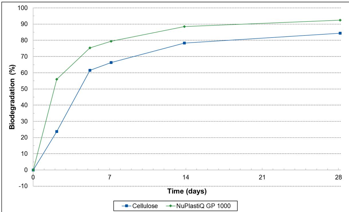
Figure 11. Evolution of the average biodegradation percentage of reference and test item (based on CO<sub>2</sub> production)
