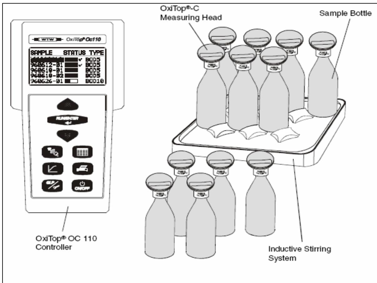
Figure 1. Set-up marine biodegradation test
