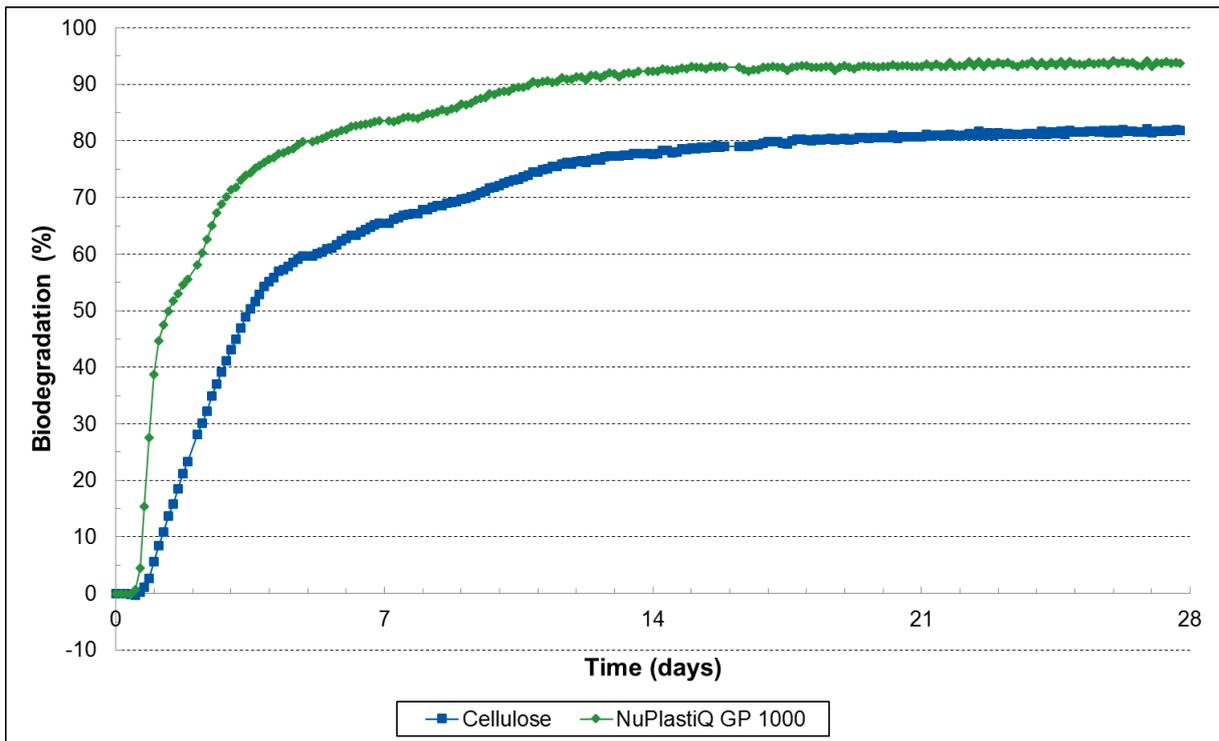
Figure 5. Evolution of the average biodegradation percentage of reference and test item (based on O<sub>2</sub> consumption)
