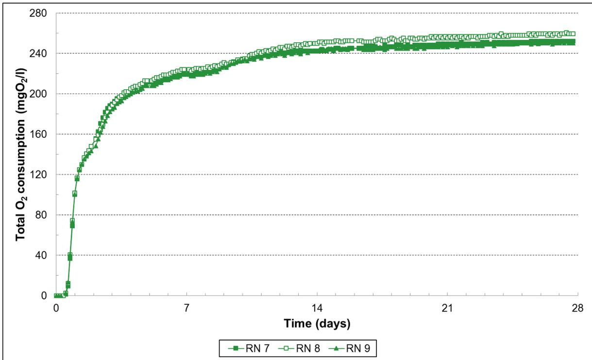
Figure 4. Evolution of the cumulative O<sub>2</sub> consumption of the NuPlastiQ GP 1000 reactors
