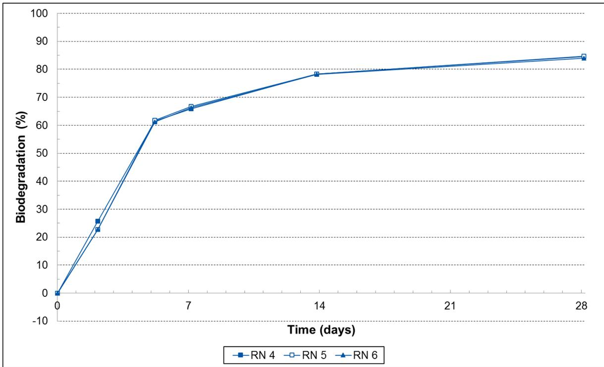
Figure 12. Evolution of the biodegradation percentage of replicates of cellulose (based on CO<sub>2</sub> production)
