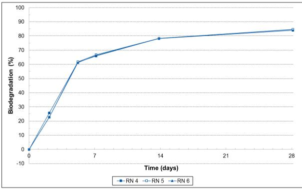
Figure 12. Evolution of the biodegradation percentage of replicates of cellulose (based on CO<sub>2</sub> production)
