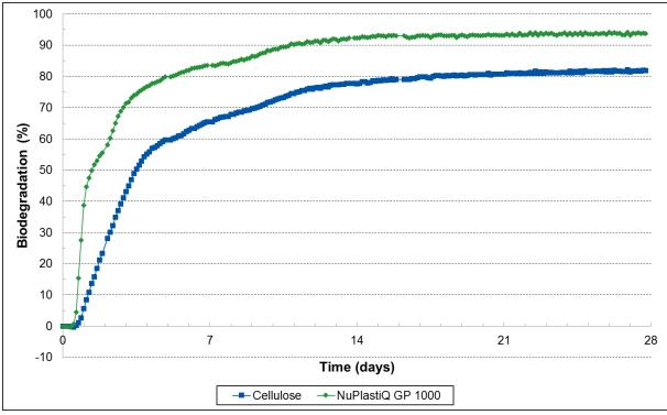
Figure 5. Evolution of the average biodegradation percentage of reference and test item (based on  $O_2$  consumption)
