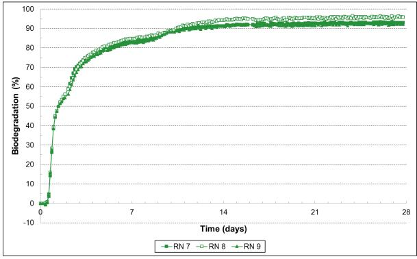
Figure 7. Evolution of the biodegradation percentage of replicates of NuPlastiQ GP 1000 (based on  $O_2$  consumption)
