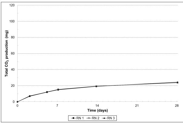
Figure 8. Evolution of the cumulative CO<sub>2</sub> production of the control reactors
