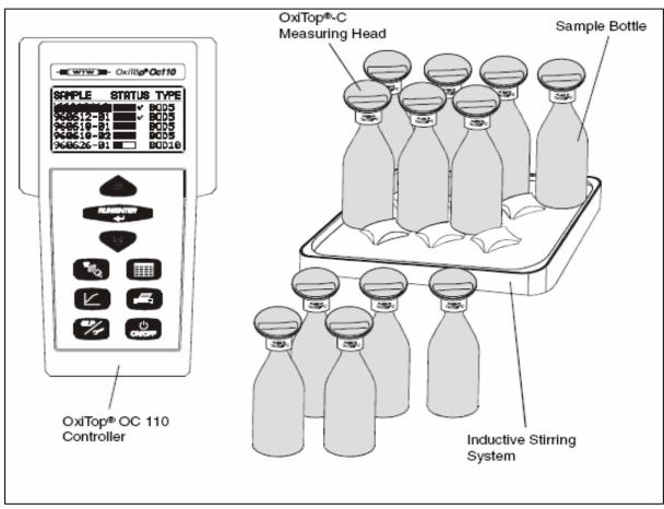
Figure 1. Set-up marine biodegradation test
