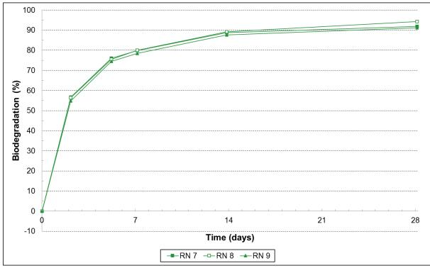
Figure 13. Evolution of the biodegradation percentage of replicates of NuPlastiQ GP 1000 (based on CO<sub>2</sub> production)
