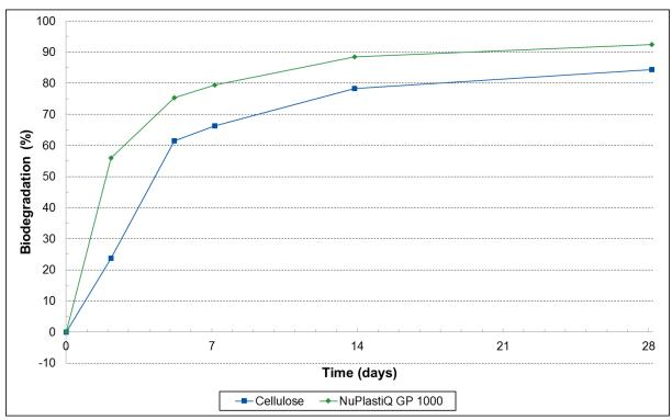
Figure 11. Evolution of the average biodegradation percentage of reference and test item (based on CO<sub>2</sub> production)
