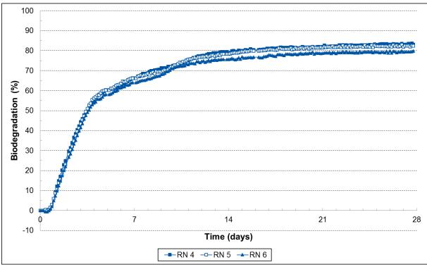
Figure 6. Evolution of the biodegradation percentage of replicates of cellulose (based on O<sub>2</sub> consumption)
