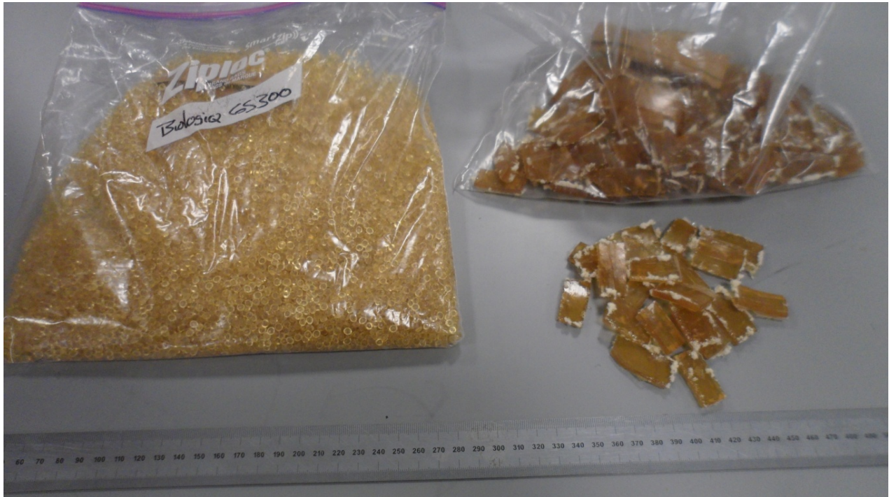
Figure 1: J-00110670 samples as received (left) and as prepared for disintegration testing (right)
